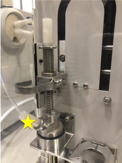
The star indicates the piece on SC1 that should be tightened after every measurement. The sample will not be able to run through the system and no data will be obtained if this is not tight after every measurement.
